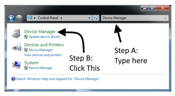
**Step 6** – Type "Device Manager" in the search field at the top right (Step A) then click on the Device Manager link that appears (Step B).
