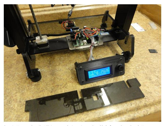
**Step 4** – You can place the LCD in a normal orientation on the table (refer to photo above). You can now access the USB port on the main circuit board. Connect your USB printer cable to this circuit board and to your PC.
