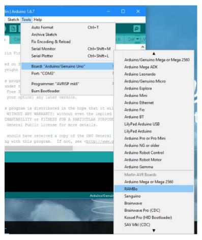
**Step 10** – Go to the Tools menu and then click on the Board option (highlighted in blue). In the menu that appears, there is a large listing of possible board types. Move your mouse cursor over the black down arrow to scroll the list down. In the list, find the RAMBo option and then left click on that.
