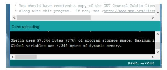
**Step 13** – When finished, the interface will state "Done Uploading." If there were any problems with the uploading procedure, a message will appear in the black area informing you of what is wrong. If any problems were encountered, you can try uploading again after selecting a different COM port in Step 11 or you can contact support.
