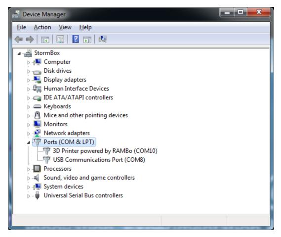
**Step 13** – You will notice that the RAMBo option has changed to say 3D Printer powered by RAMBo. This indicates that the printer's driver has successfully installed and you are ready to flash.
