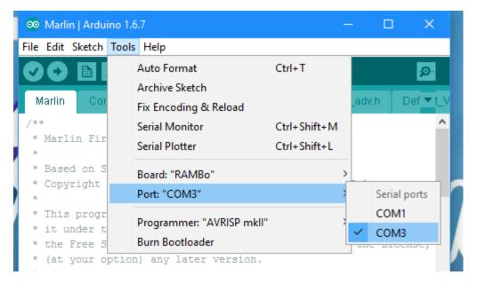
**Step 11** – Go to the Tools menu and then left click on the Port option (highlighted in blue). A list of COM ports are shown on the screen, in most cases there is only one choice you can make. If you have multiple choices, the bottom choice is usually the correct choice (if things don't work later on then repeat this step and select a different choice). Select the COM port for your printer by left clicking on it.
