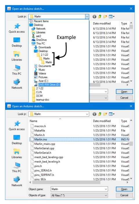
**Step 8** – Navigate into the folder that was previously extracted (similar to 2.1-22) then the Marlin folder then the Marlin folder again (shown in top photo). Open the Marlin.ino file (shown in bottom photo) by left clicking on it once then clicking on Open.
