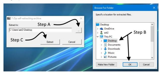
**Step 3** – Click on the ... button to the right of the Extract to: location (Step A), select a location to extract the files to (we recommend the Desktop) and then click OK (Step B), then click Extract to extract the files to that location (Step C).
