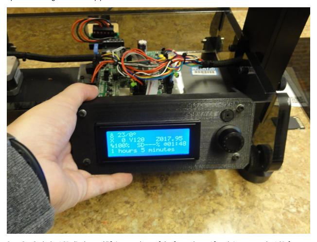
**Step 2** – Grab the LCD display and lift it up and out of the front plate. After doing so, set the LCD face down on the table.
