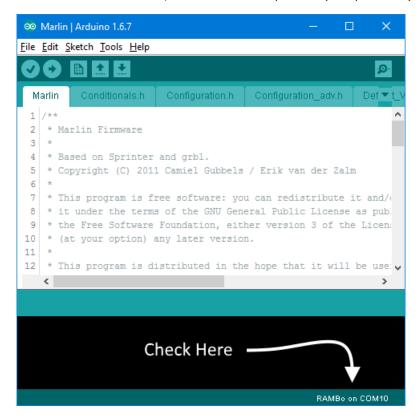
**Step 10** – Verify that the correct board (RAMBo) and correct COM port is selected in the main interface, these options should match what you selected in the prior 2 steps.
