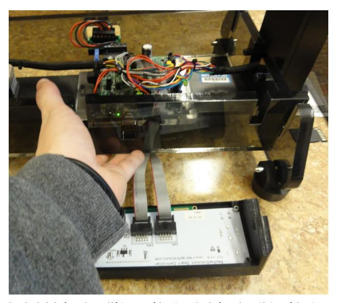
**Step 3** – Grab the front plate and lift it up out of the printer. Set the front plate aside in a safe location.
