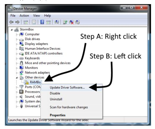
**Step 7** – Find the RAMBo device in Other Devices and right click on it (Step A). In the menu, left click on Update Driver Software... (Step B).
