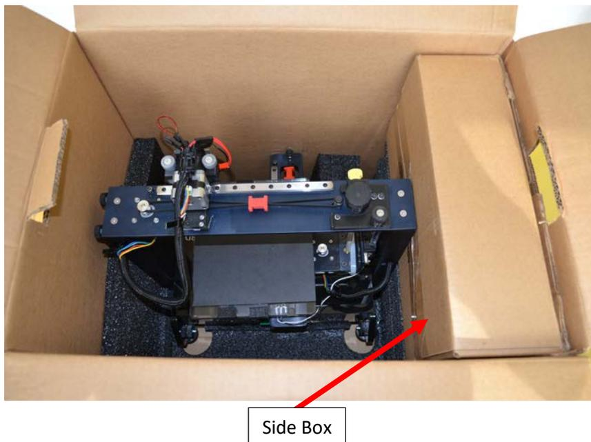
3. By grabbing both sides of the printer frame, lift the printer out of the box
